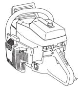
Clean the cooling system with a brush once a week, more often in demanding conditions. A dirty or blocked cooling system results in the machine overheating which causes damage to the piston and cylinder.
